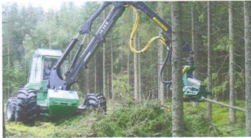
The most obvious innovative feature of the new T-Bear harvester; adjustable track width from 2.9 to 3.5 metres at the touch of a button. Photo: Pellewood
